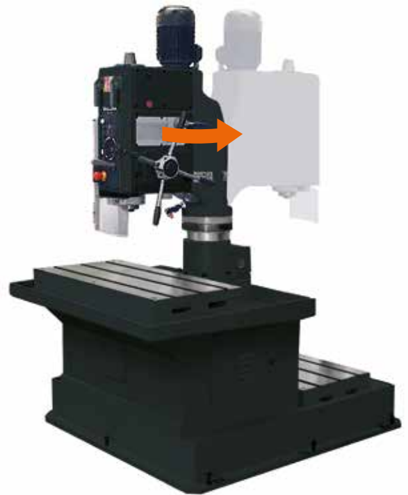
Drilling with a rotating head on a double table bench. The lower rear table enables work on bulky parts.
