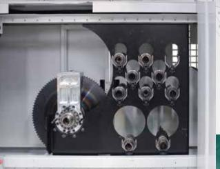
The new XBLADE CNC line is capable of processing steel construction beams of different sizes, with sections up to 305x305 on three sides, 450x450 on one side and variable lengths thanks to its modular configuration.
