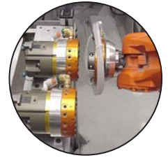
Quick Change Grippers for Automatic Change between Parts
