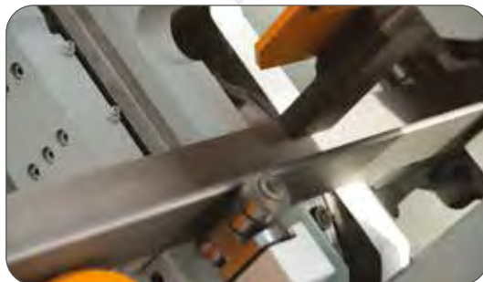
A CNC marking press can be provided to generate the required part number without any character set up.
