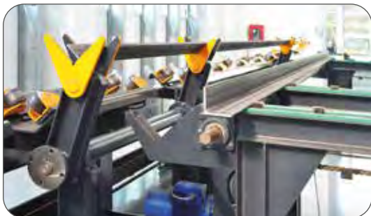
A stock length material transfer table with rotary loader can automatically index and load the next stock length as required.
