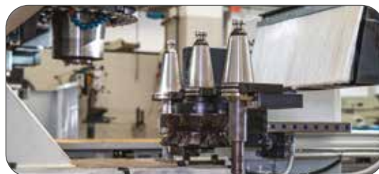
Automatic 5-position tool changer on each side (6 positions available upon request)
