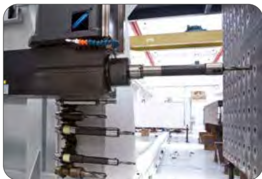
Horizontal spindle with automatic tool changer
