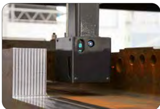
Non-contact triple laser probing
