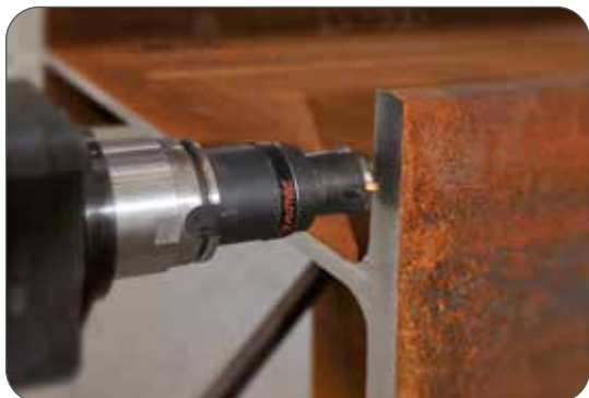
Rotating drilling head for end milling
