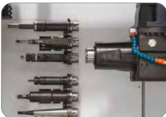
Automatic tool changer with 9 positions
