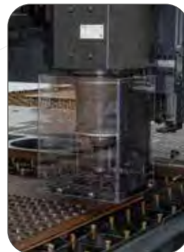
Drilling unit with a 6-position automatic tool changer
