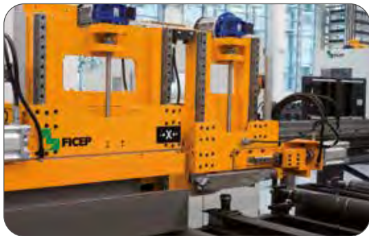
Second positioning arm for reduced overall dimensions
