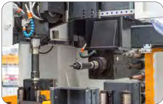
Optional second drill head with automatic tool changer
