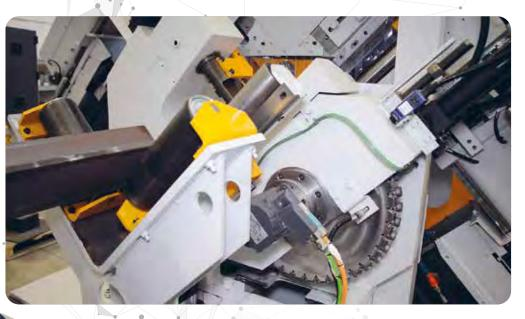
Angles with full miter cuts on both ends can be processed to generate typical framing structures. The versatility of processing flats up to 20" x 1" is exhibited with its ability to not only cut the part to length but also clip the corners as required.
