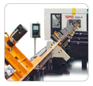
Stock material positioning and measuring into the TIPO D50-F is accomplished with a positive rack and pinion system. Once the clamping of the material is confirmed, the stock length is automatically measured prior to the start of the fabrication process.
