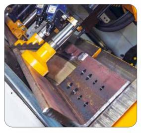
The TIPO D50-F includes a miter-cutting circular saw with carbide inserts for maximum productivity. The saw can position automatically for miter cuts of up to  $60^{\circ}$  in either direction.
