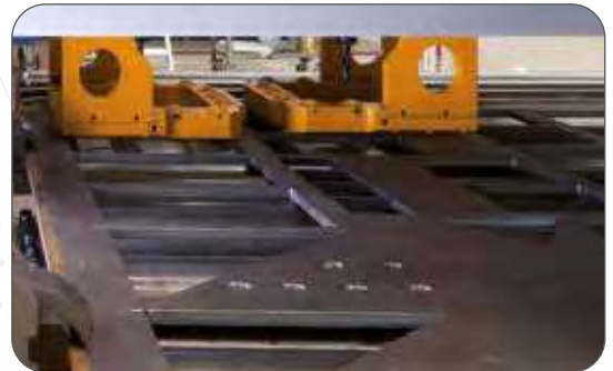
Hold-downs and material upholding supports
