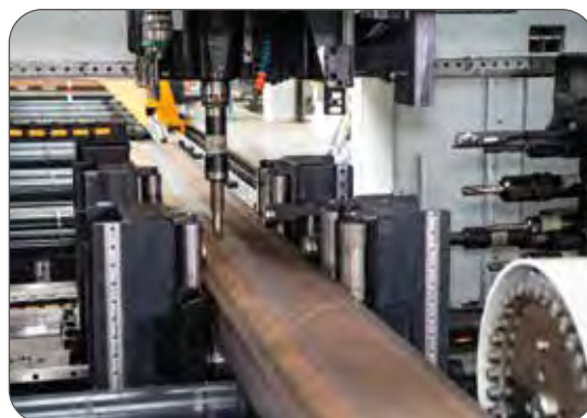
6-position automatic tool changer
