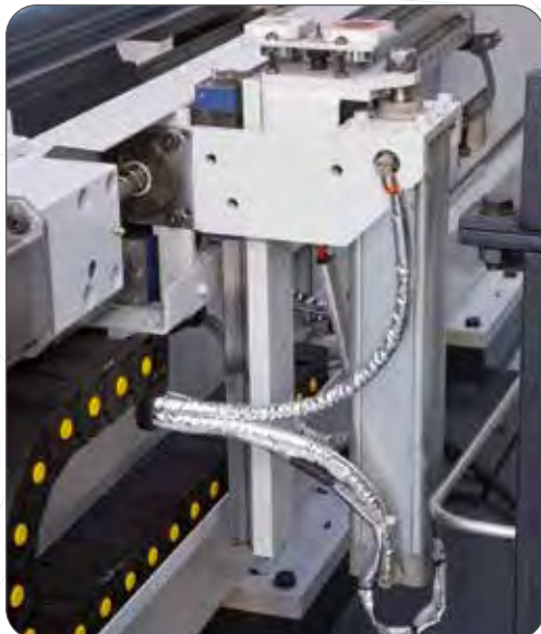
Underside web scribing device
