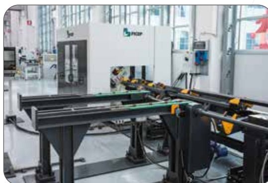
Infeed cross transfer and rotating loading system
