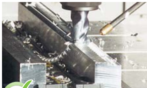
Machining with MQL
