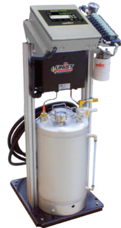
Auto refill fluid supply system incorporates a 10 gallon [38 liter] ASME-rated stainless-steel pressure tank with 0–60 psi [0–4 bar] precision regulator and integral high and low level switches. The system also includes PLC controls and an electric pump to automatically refill the tank, which eliminates downtime. This system provides superior performance when drawing fluid from a tote or drum.
