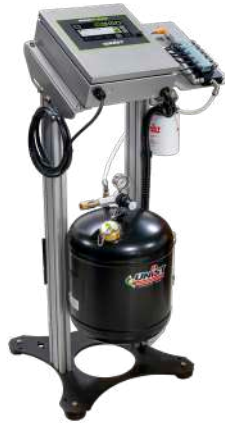
6 gallon [22 liter] ASME-rated pressure tank comes equipped with a 0–100 psi [0–7 bar] regulator, low level switch and sight gauge.
