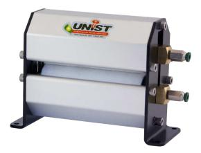
The lubricant is transferred to the stock through durable polyester felt or polyurethane foam roller covers. These cover materials apply the lubricant smoothly and evenly across both sides of the stock.
